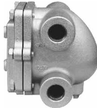
At the top of the trap is a thermostatic air vent that discharges all air and noncondensable gases as soon as they reach the trap. This allows for maximum condensate drainage. The air vent reacts to the system temperature and will close at a temperature a few degrees below saturation to prevent steam leakage. A drain plug is located at the bottom of the trap body to permit easy flushing of dirt.
